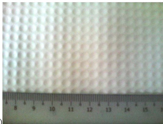
Figure 1. (a) Perforated aluminium support embedded in the permeate compartment which is used to support the membrane during VMD. (b) Dimples stamped over the PVDF membrane surface after the VMD process.
