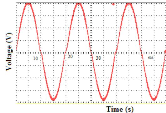
Figure 8. Inverter output voltage waveform after filtering.
