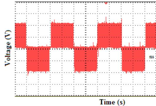
Figure 7. Inverter output voltage waveform before filtering.
