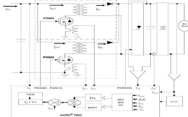
Figure 3. Measurement of grid voltage required for PLL.
