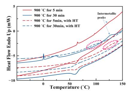
Figure 6. Differential Scanning Calorimeter (DSC) curves of Ti-51%Ni SMAs sintered at 900°C for 5 and 30 min. with and without homogenization heat treatment.
