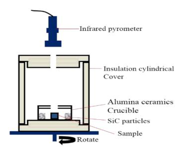
**Figure 1.** Schematic diagram of MWS insulation barrel.
