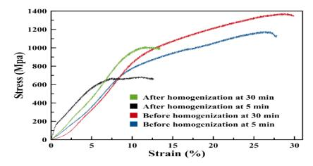
**Figure 5.** Compression curves of Ti-51%Ni SMAs sintered at 900°C.
