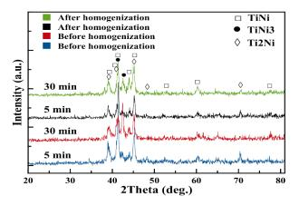
**Figure 4.** XRD patterns of Ti-51%Ni SMAs sintered at 900°C.
