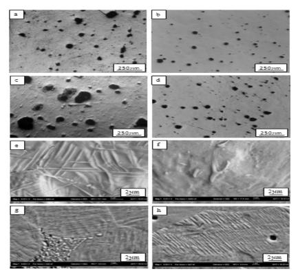
Figure 2. Field Emission Scanning Electron Microscopy (FESEM) and optical micrographs of Ti-51%Ni Shape Memory Alloys sintered at 90 °C for (a and e) 5 min, (b and f) 30 min, (c and g) 5 min, followed by HT at 900°C for 30 min. and water quenching and (d and h) 30 min, followed by HT at 900°C for 30 min and water quenching.
