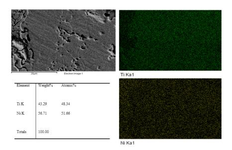
**Figure 3.** Mapping of Ti-51%Ni SMA sintered at 900°C for 5 min. after HT at 900°C for 30 min. and water quenching.
