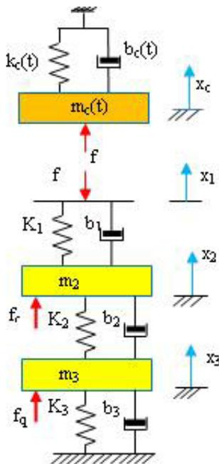
**Figure 3.** The model of the pantograph-catenary interaction.
