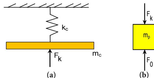
**Figure 1(a).** The catenary model. **(b).** The pantograph model.
