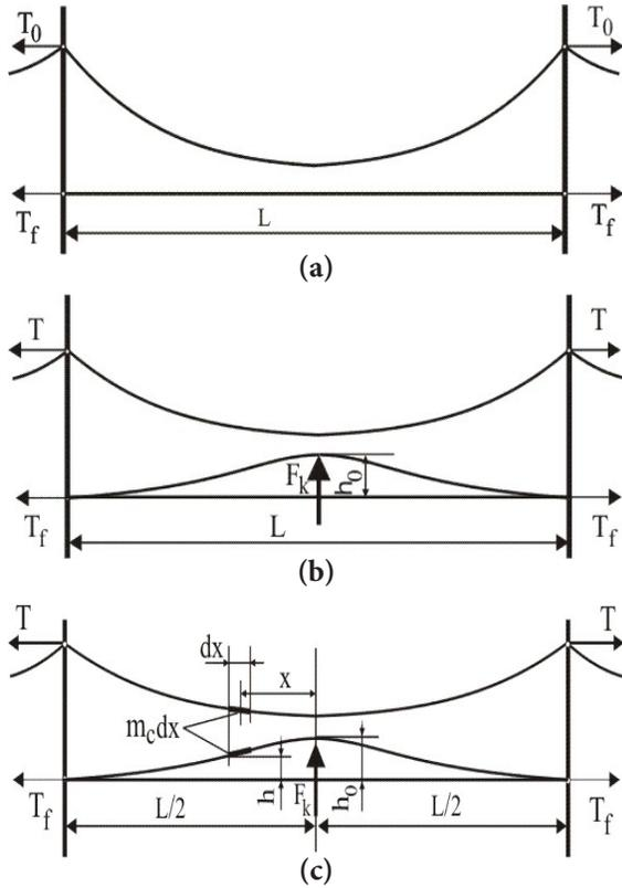
**Figure 2.** The forces acting on the catenary. (a) The catenary at standstill. (b) The shape of the catenary when the pantograph is on the middle of the span. (c) Catenary analysis for a distance  $x$  from the middle of the span.
