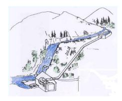
Figure 10. Scheme of the damless sleeve mini-hydroelectric power station<sup>21</sup>.
