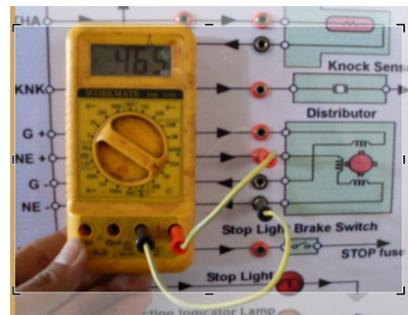
Figure 24. Ne Sensor Resistance Check.
