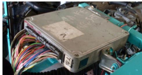
Figure 9. Engine ECU with Original Wiring Harness.
