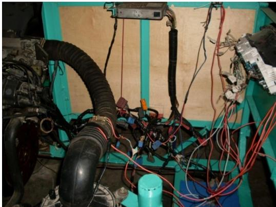
**Figure 6.** SSB Wiring Harness and Connectors.
