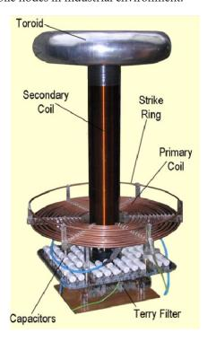
Figure 1. Tesla coil.
