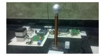
**Figure 5.** ABBA resonant power transmission using Tesla coil.
