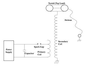
Figure 3. Block diagram of Tesla coil.
