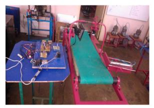
**Figure 2.** Photo image of the on line inspection for machine vision process.
