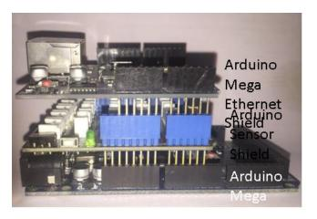
Figure 1. Arduino Mega 2560 node – prototype model.
