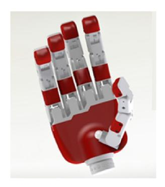
Figure 3. The three-dimensional model of the manipulator in solidworks (CAD).
