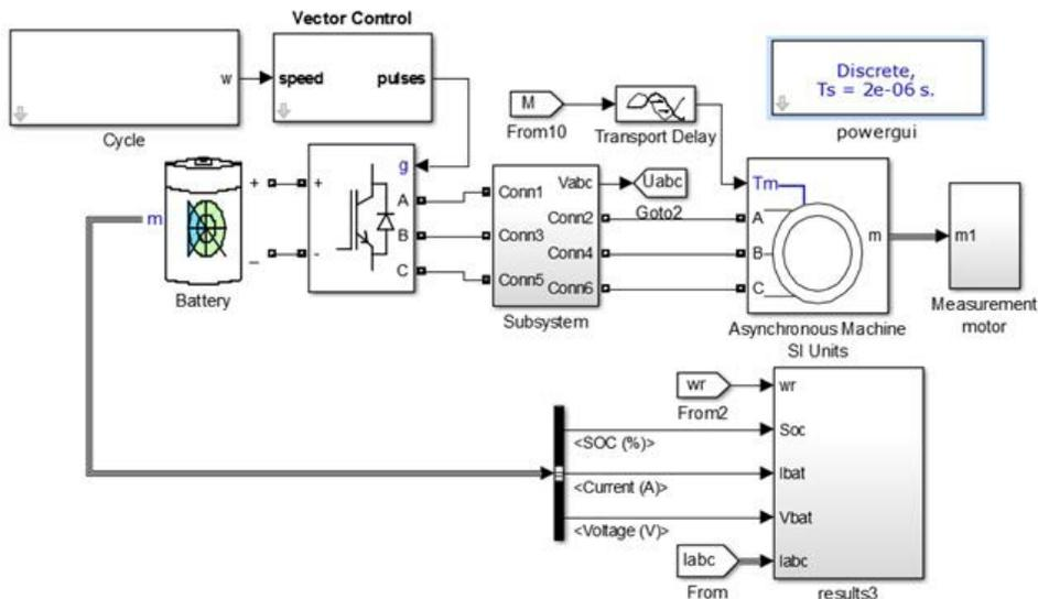
Figure 4. Mathematical model of system with IM in simulink software.
