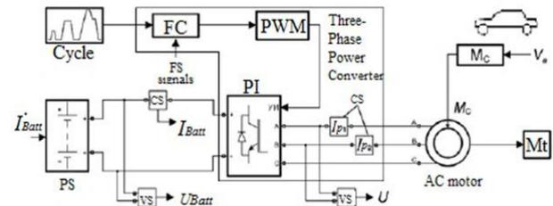
**Figure 1.** Flow sheet of comprehensive mathematical model of electric vehicle.
