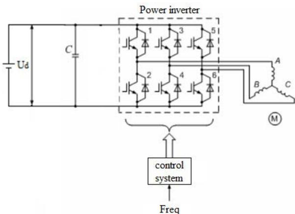
Figure 8. Structure of frequency converter with DC source and controlled amplifier.
