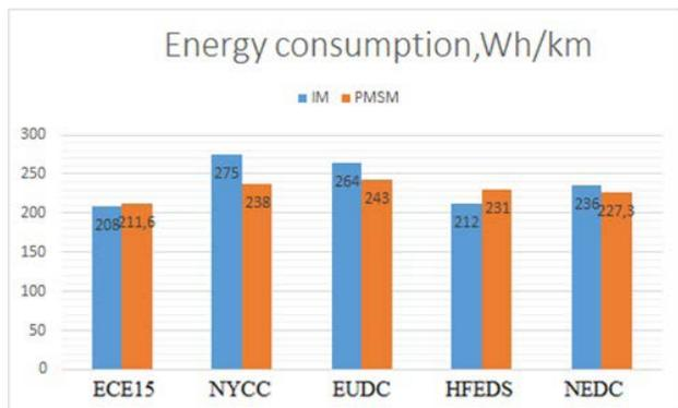
**Figure 19.** Specific energy consumption in cycles for two systems, taking into account for regeneration.
