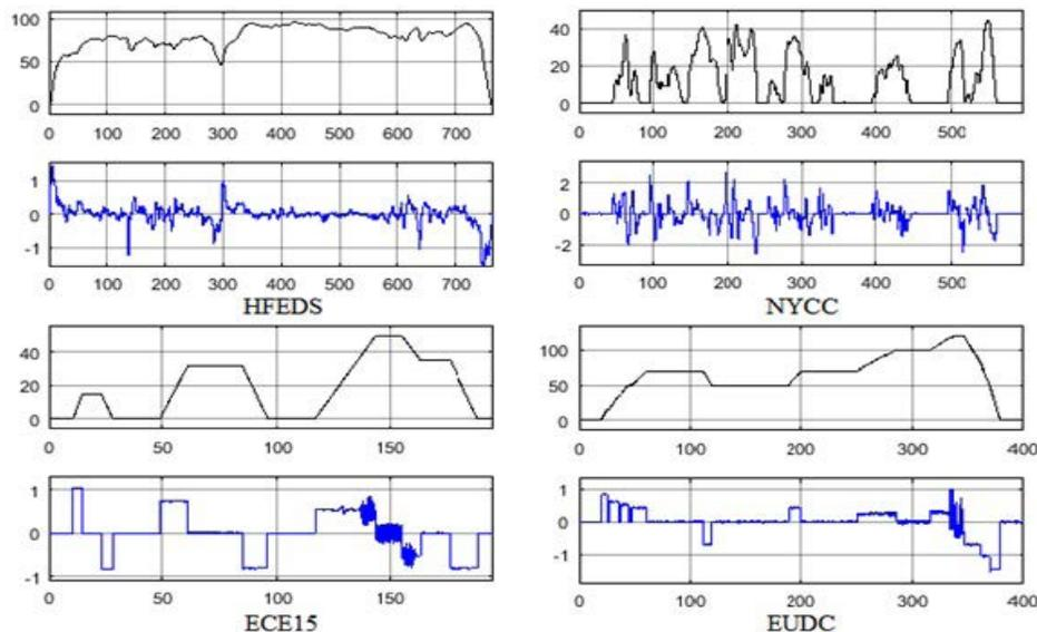
Figure 16. Speed and acceleration in cycles: ---- acceleration; ---- speed.
