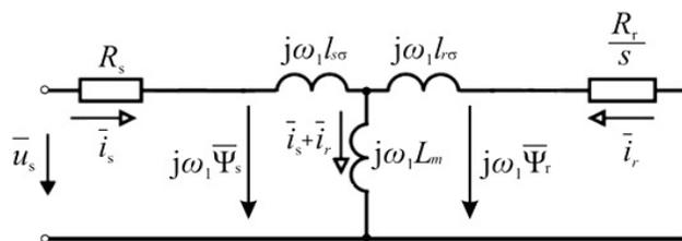
Figure 2. Equivalent circuit of asynchronous machine.
