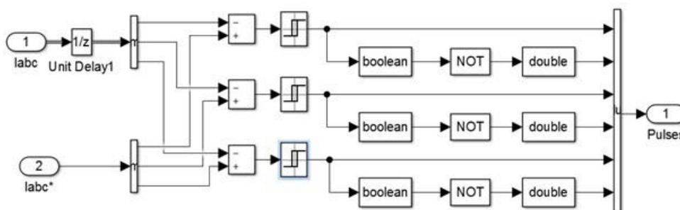
Figure 15. Implementation of current relay circuit in simulink software.
