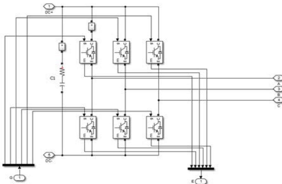
Figure 9. Mathematical model of traction inverter in simulink software.
