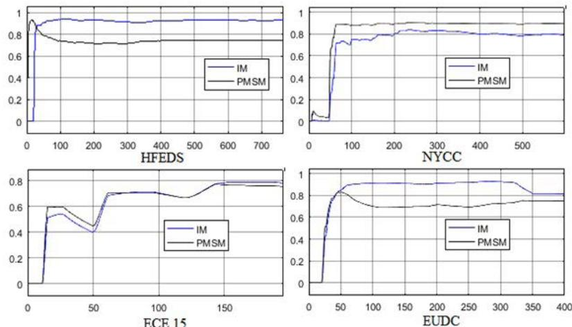
**Figure 18.** System efficiency in cycles.
