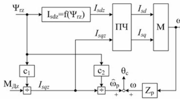
Figure 12. Drive structure with indirect orientation by field.
