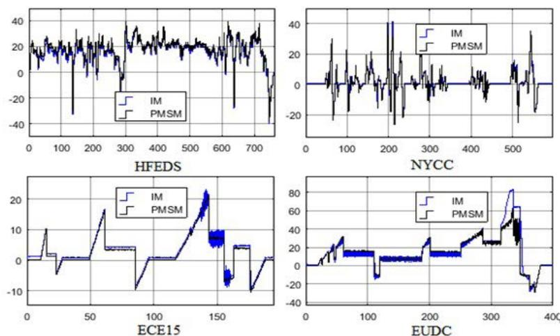
**Figure 17.** Consumed power of electric motor in cycles.
