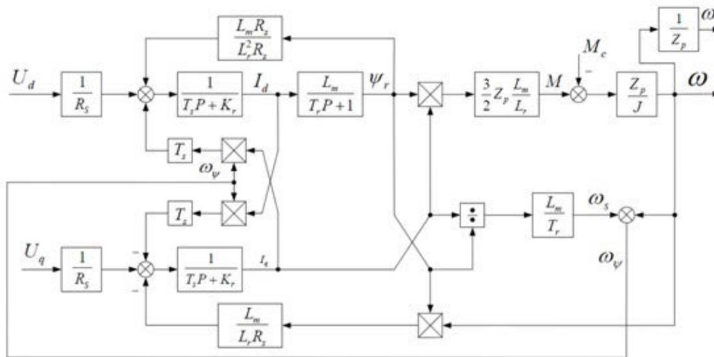
Figure 3. Structural diagram of asynchronous machine in coordinates (d, q).
