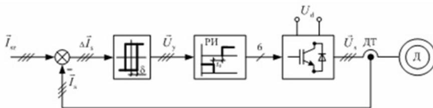
Figure 14. Structural diagram of current relay circuit.
