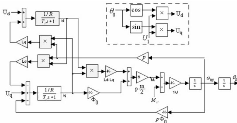
Figure 5. Structural diagram of motor in fixed coordinate system.
