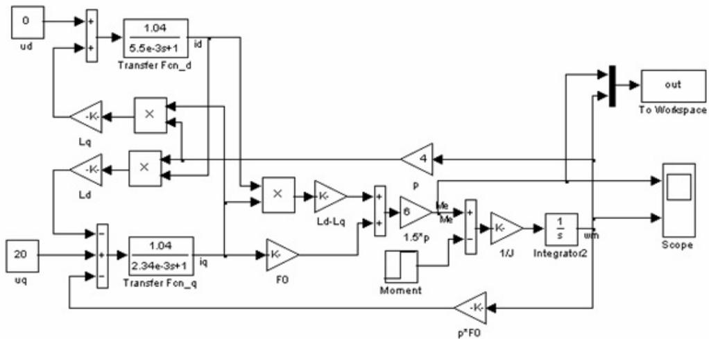
Figure 6. Mathematical model of motor in rotation coordinate system.
