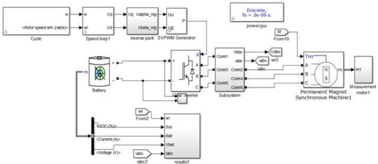
Figure 7. Mathematical model of system with PMSM motor in simulink software.
