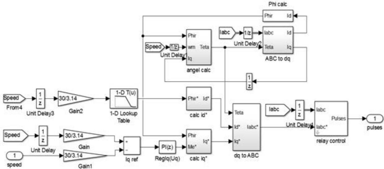
Figure 13. Control system of IM in simulink software.
