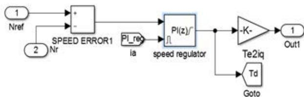
Figure 11. Subsystem of speed control unit.
