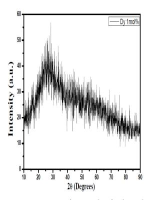
**Figure 1.** XRD spectrum for 1.0 mol% of Dy<sup>3+</sup> ion doped calcium sulfo borophosphate glasses.
