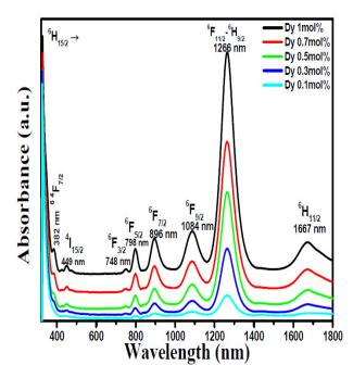
**Figure 2.** Absorption spectrum of calcium sulfoborophosphate doped Dy<sup>3+</sup> glasses.
