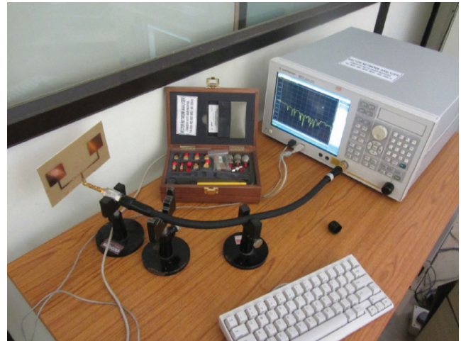
Figure 10. Experimental set up for measuring the characteristics parameters of microstrip patch antenna array.
