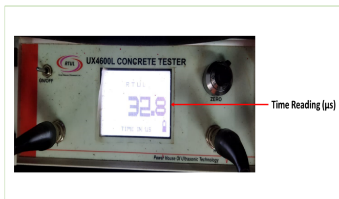
Fig 5. Display of UPV test set up
