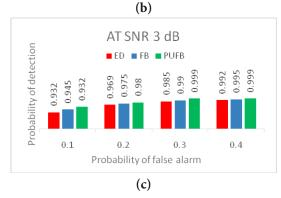
**Figure 7.** Performance of spectrum sensing techniques over AWGN channel at different SNR values.
