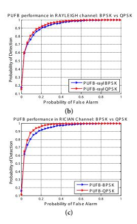
**Figure 10.** Comparative ROC curves for FB sensing techniques with BPSK and QPSK modulation techniques.
