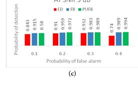
**Figure 8.** Performance of spectrum sensing techniques over RAYLEIGH channel at different SNR values.
