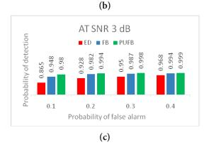
**Figure 9.** Performance of sensing techniques over RICIAN channel at different SNR.
