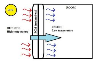
Figure 1. Schematic Diagram Working of PCM.
