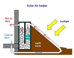
Figure 4. Schematic Diagram of Active Technology.
