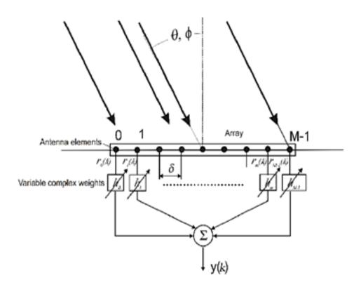
**Figure 1.** Uniform Linear antenna array geometry.
