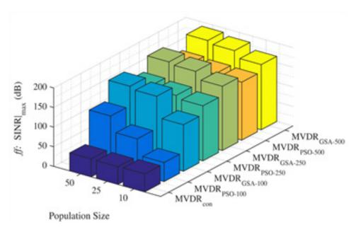
Figure 4. Performance comparison of average SINR for optimized MVDR<sub>PSO</sub> and  $MVDR_{GSA}$ .
