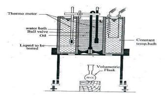
Figure 1. Redwood Viscometer<sup>13</sup>.
