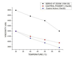
Figure 4. Temperature viscosity graph.
