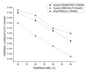
Figure 6. Temperature thermal conductivity graph.
