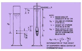
Figure 2. Hydrometer 14.
