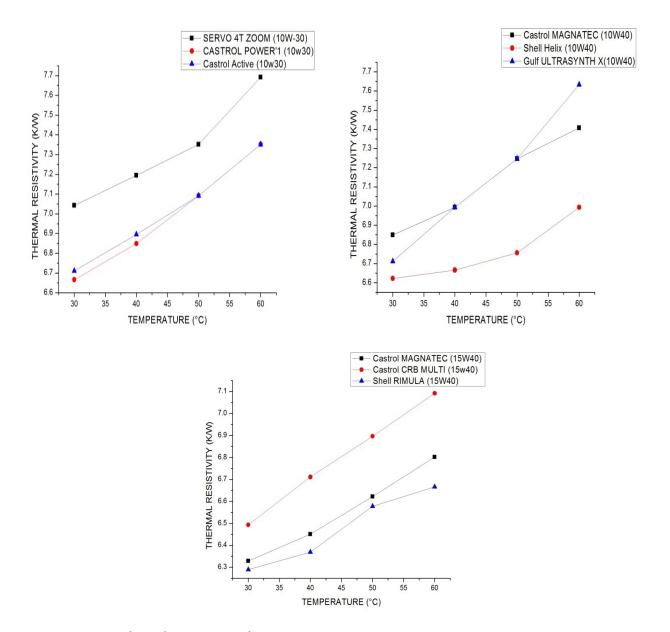
Figure 7. Temperature thermal resistivity graph.
