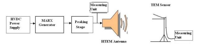
Figure 1. Block diagram of electromagnetic field generator.
