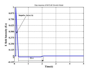
Figure 4(b). Radiated output pulse for step input pulse.
