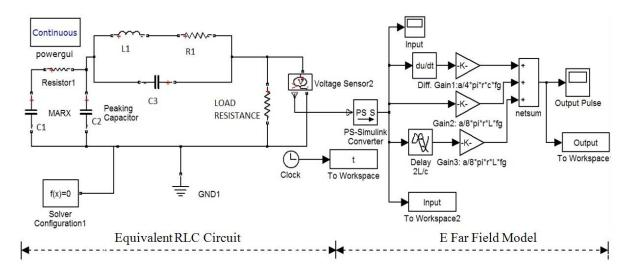
Figure 3. The RLC modelling for the far field radiation.
