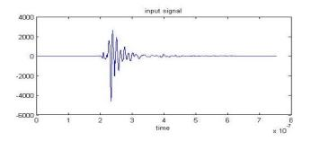
**Figure 9(a).** Time-amplitude representation of the radiated E far field - 4.9 kV/m.
