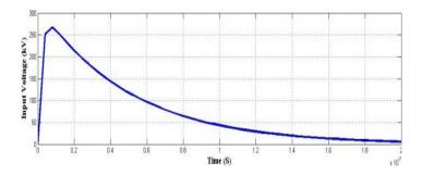
Figure 5(a). Exponential decaying input pulse.
