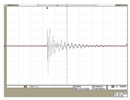
Figure 8. The E far field amplitude is 14.4 kV/m
