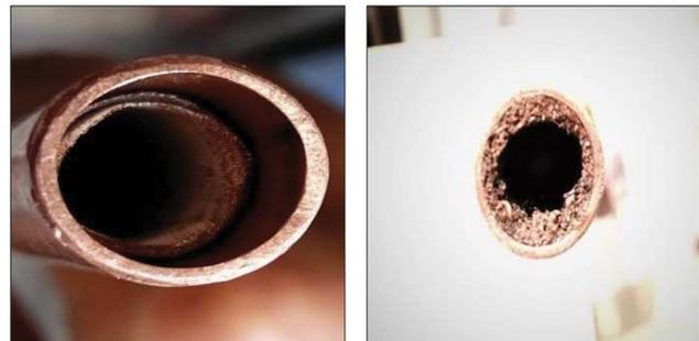
Figure 2. Cross-sectional view of sintered and mesh wick heat pipes.
