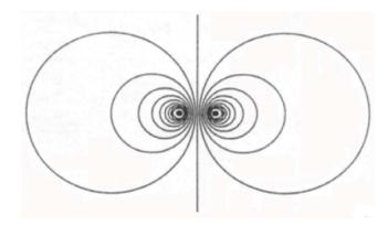
Figure 1. Electrical field lines generated by probe configuration.
