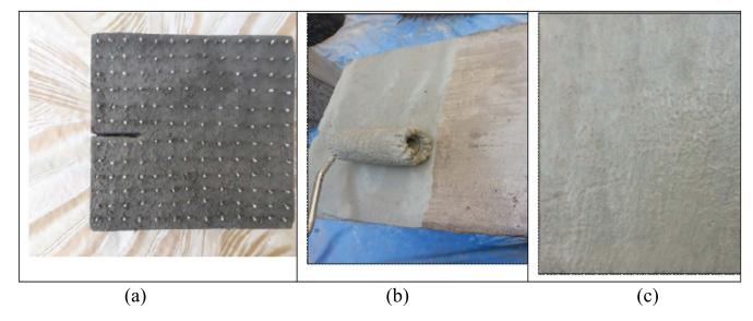
Figure 4. Preparation of specimens (a) Creation of crack (b) Coating with epoxy (c) Final-finished of specimens.
