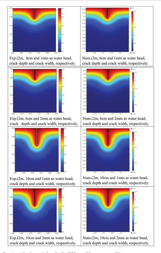
Figure 13. Experimental and numerical results after 312 hours of the exposure conditions
