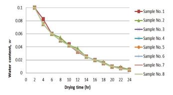
**Figure 7.** Oven drying and water content change of calibration samples.
