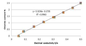
**Figure 9.** Electrical conductivity verse chloride contents.
