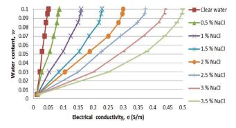
**Figure 8.** Relationship between chloride contents and electrical conductivities.
