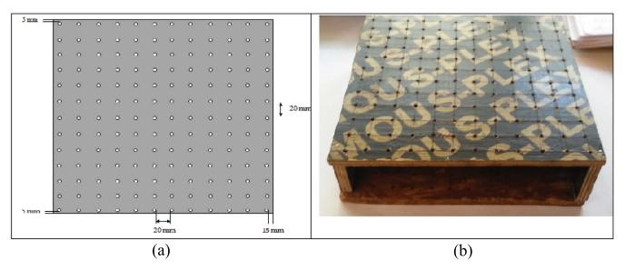
Figure 3. Double-layered probe holder, (a) Schematic representation with dimensions. (b) Picture of an actual holder.
