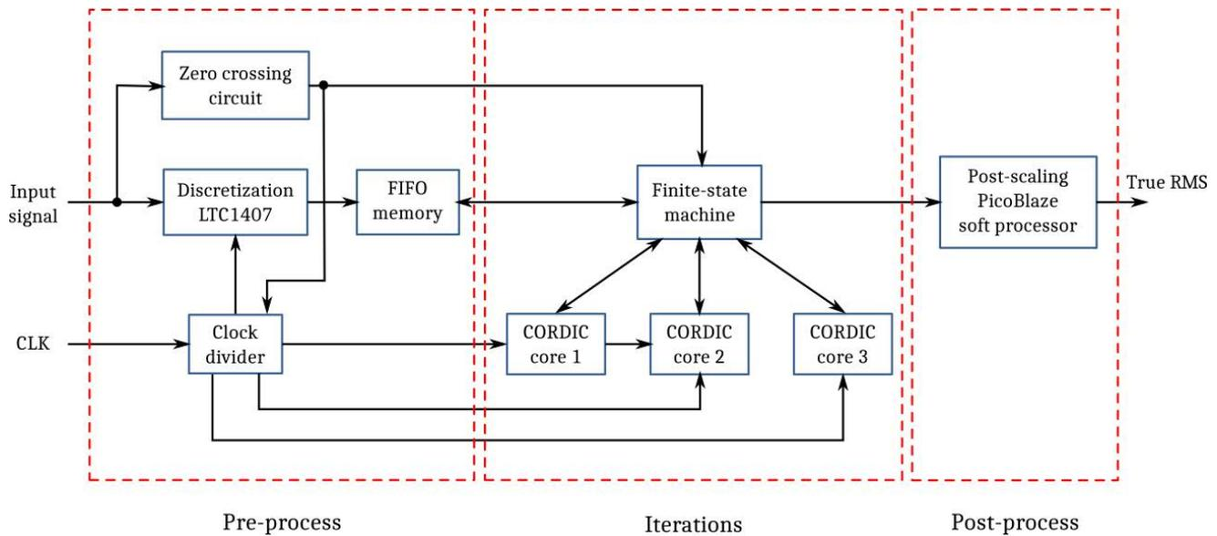
Figure 2. Hardware architecture.
