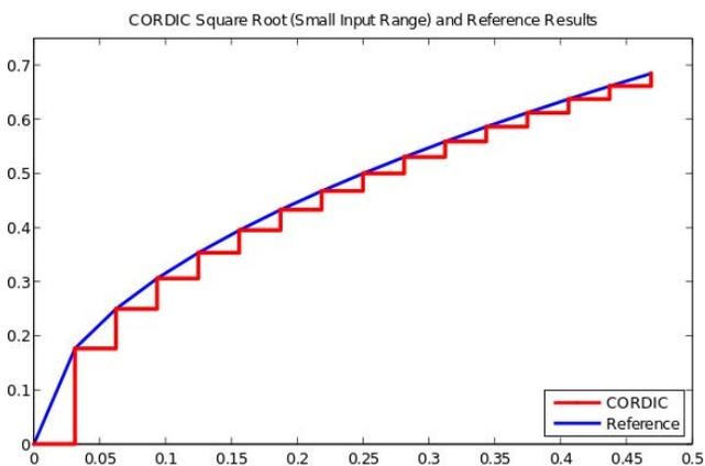
Figure 4. Computer simulation vs CORDIC implementation result of the square root function.
