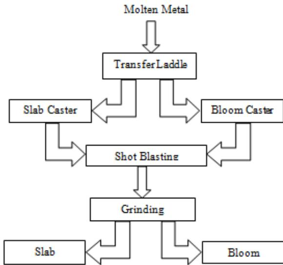
Figure 1. Flow chart of the casting process.
