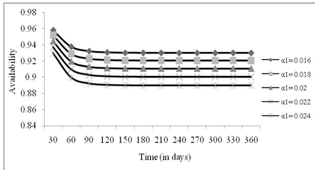
Figure 3. Effect of failure rate of transfer laddle on availability.
