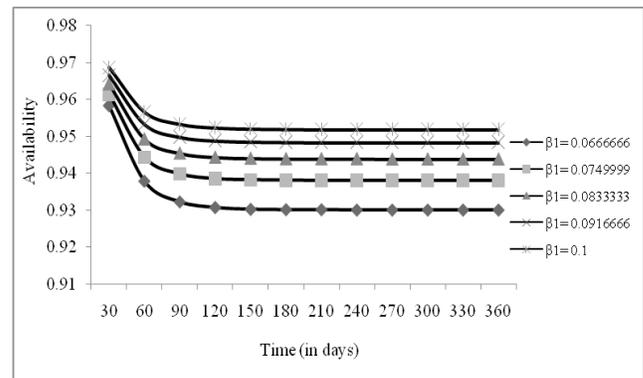
Figure 4. Effect of repair rate of transfer laddle on availability.
