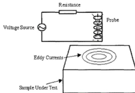
**Figure 1.** Principle for Eddy Currents.
