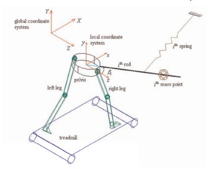
**Figure 1.** The 3D schematic of the passive device connected to pelvis.
