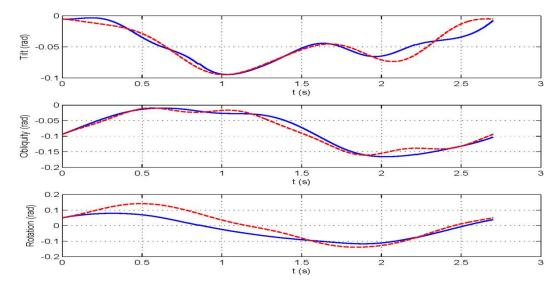
**Figure 5.** Tilt, Obliquity and Rotation trajectories of pelvis of subject during gait cycle for case (A). Solid blue lines: Actual Trajectories, Dashed red lines: Desired Trajectories.
