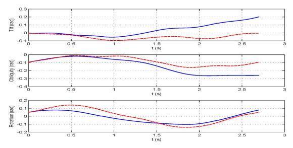
**Figure 8.** Tilt, Obliquity and Rotation trajectories of pelvis of subject during gait cycle by variation of design parameters. Solid blue lines: Actual Trajectories, Dashed red lines: Desired Trajectories.
