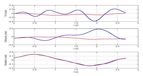
**Figure 7.** Rotation trajectory of pelvis of subject during gait cycle for case (C). Solid blue line: Actual Trajectory, Dashed red line: Desired Trajectory.
