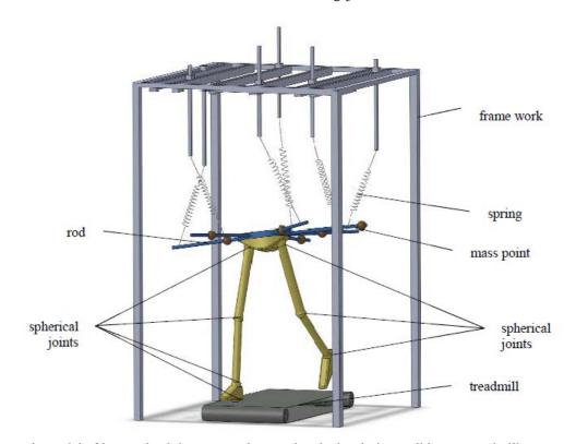
**Figure 3.** Dynamic model of legs and pelvis connected to passive device during walking on treadmill.
