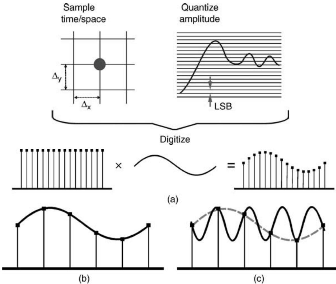
Figure 4. Digitization, sampling, quantization and aliasing explanation.
