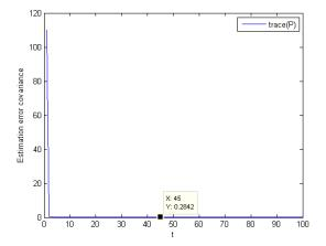
**Figure 9.** Trace of estimation error covariance matrix ( $\sigma^2 = 0.5^2$ ).
