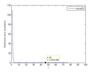
**Figure 5.** Trace of estimation error covariance matrix ( $\sigma^2 = 0$ ).
