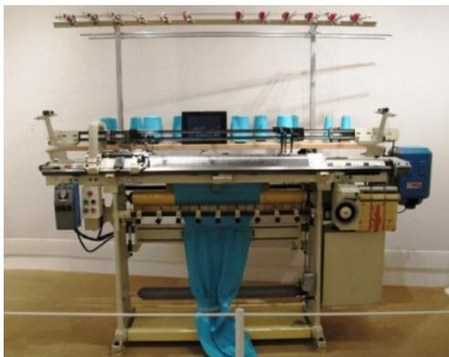
Figure 2. Computerized flat knitting systems.
