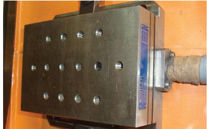
**Figure 3.** Close-up view of Dynamometer.
