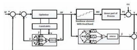
Figure 7. A RBF neural network model can be incorporated into linear model predictive control scheme.
