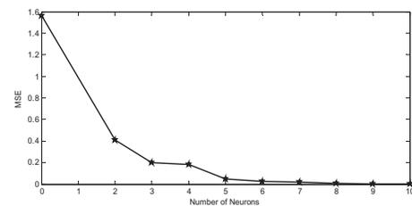
Figure 6. Performance of RBF neural network based model on number of neurons in hidden layer.
