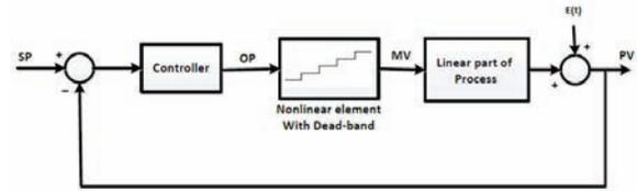
Figure 1. Process control loop in the presence of dead-band.
