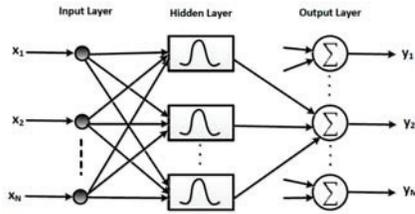
**Figure 2.** Structure of a radial basis function (RBF) neural network.
