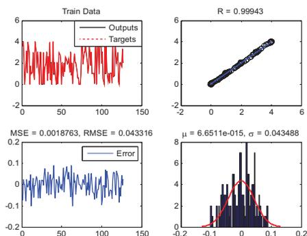
Figure 4. Performance of RBF neural network based model on sets of training data.
