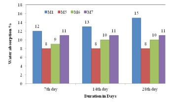
**Figure 5.** Water absorption comparison of FaL-G and QuFaL-G bricks.
