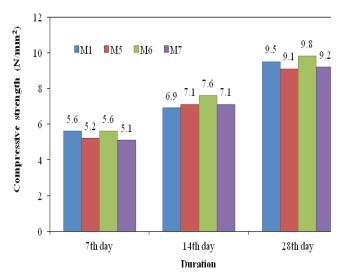
**Figure 3.** Compressive strength comparison of FaL-G and QuFaL-G bricks.
