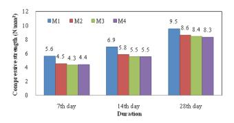
**Figure 1.** Compressive strength of FaL-G bricks.
