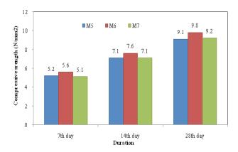
Figure 2. Compressive strength of QuFaL-G bricks.
