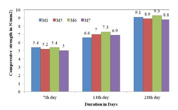
**Figure 4.** Compressive strength comparison of FaL-G and QuFaL-G Bricks after sulphate intrusion.
