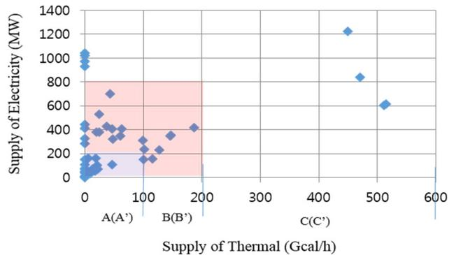
**Figure 6.** Classification of IEB depending on heat and electricity supply capacity.
