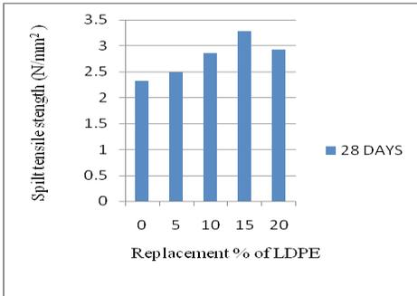
Figure 6. Split Tensile strength of specimen.
