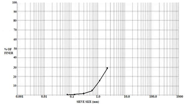
**Figure 4.** Particle size distribution for pulverized LDPE plastic waste.
