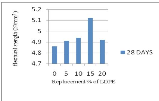
Figure 7. Flexural Strength of specimen.
