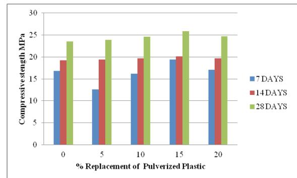
**Figure 5.** Compressive strength vs % replacement of pulverized plastic.
