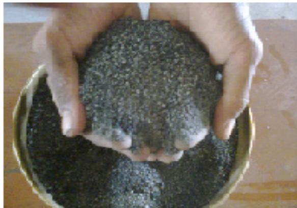
**Figure 3.** Pulverized burned LDPE fine aggregate.
