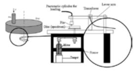
Figure 13. A scheme of pin on disk test machine.
