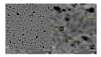
Figure 28. The microstructure of the processed area in the sample containing amplifier particles in the fourth tool pass. A) Stir area with a magnification of 10kx B) Stir area with a magnification of 75kx.
