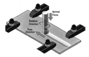
**Figure 4.** A pattern of the clamping work piece in friction stir processing.
