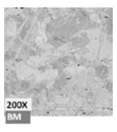
**Figure 16.** Base metal microstructure at a magnification of 200 times.
