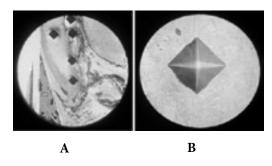
**Figure 12.** Observed images of Vickers device microscope A) The indenter effect with 200 times magnification B) The indenter effect with a 100 times magnification.
