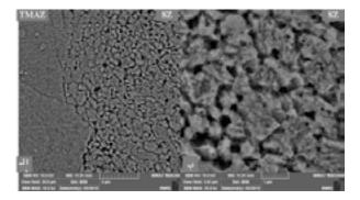
Figure 24. The microstructure of processed area in the sample without amplifier particles in the second tool pass. A) Stir areas and affected by thermo-mechanical B) Stir area.
