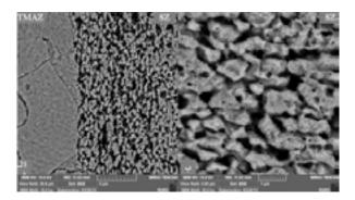
Figure 25. The microstructure of processed area in the sample without amplifier particles in the fourth tool pass. A) Stir areas and affected by thermo-mechanical B) Stir area.
