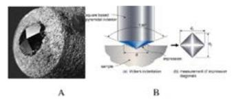
Figure 9. A picture of indentor and its effect on the Vickers test. A) A grandiosity picture of indentor B) A scheme of indentor effect in the sample.
