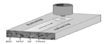
Figure 2. Different microstructure zones in friction stir processed piece.
