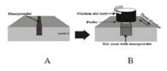
**Figure 1.** The overall picture offriction stir processing A) The seam filled with amplifier nanoparticles.
