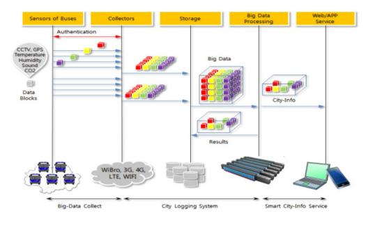
Figure 1. Composition of a city-logging system using mobile observation equipment.
