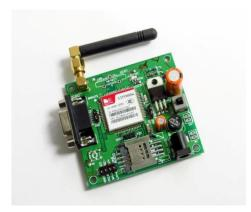
Figure 3. GSM module.
