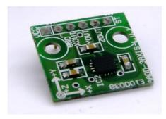
Figure 2. Accelerometer sensor.
