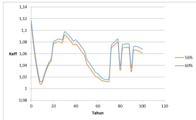
**Figure 4.** K-eff change with time during MCANDLE start-up simulation case A 1150 MWt.
