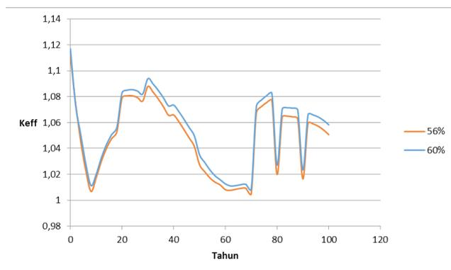
**Figure 5.** K-eff change with time during MCANDLE start-up simulation case B 1250 MWt.
