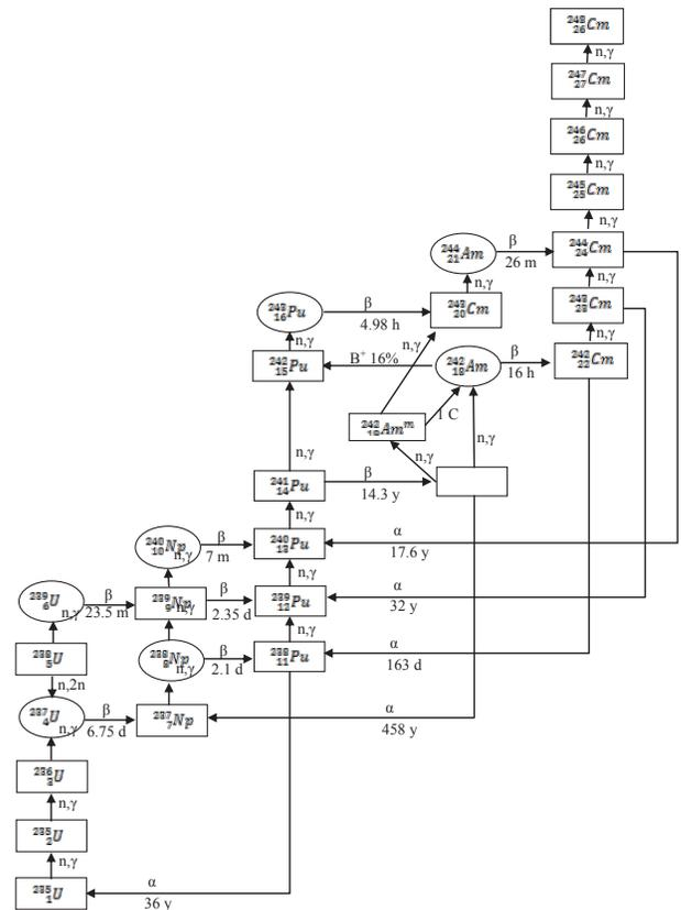
Figure 3. Nuclear Burn-up chain used in this study.
