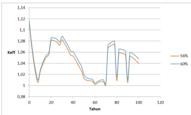
**Figure 6.** K-eff change with time during MCANDLE start-up simulation case C 1350 MWt.
