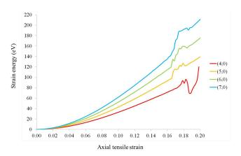
**Figure 3.** Comparison between strain energy curves of zigzag SWCNTs for (4,0), (5,0), (6,0) and (7,0) under axial tensile.
