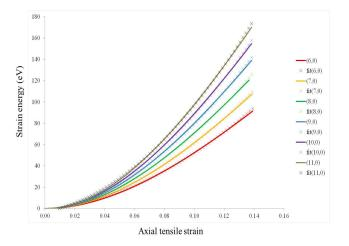
**Figure 4.** Curve fitting strain energy curves by using predicting parameters.
