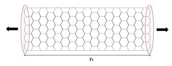
**Figure 2.** Two-dimensional view for the SWCNT under axial tension.
