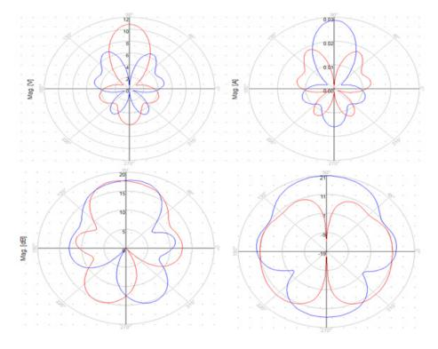
Figure 9. E-plane and H-plane polarization, circular polarization and linear polarization for 3rd itereation at 3.5 GHz.
