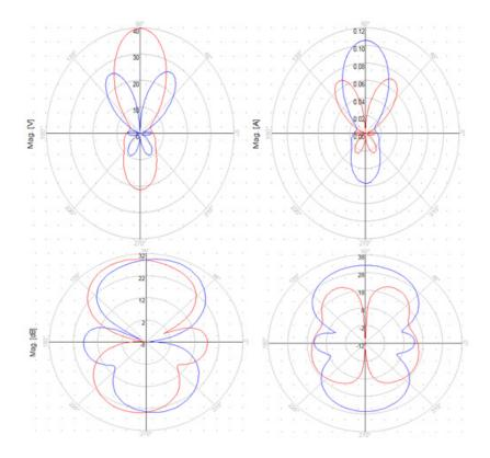
Figure 8. E-plane and H-plane polarization, circular polarization and linear polarization for 2nd itereation at 3.52 GHz.
