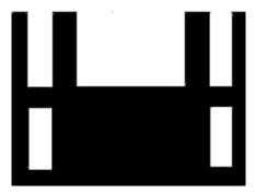
Figure 3. Antenna geometry for 2nd iteration.
