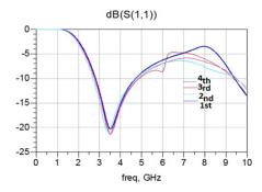
**Figure 6.** Return loss comparison for three iterations.
