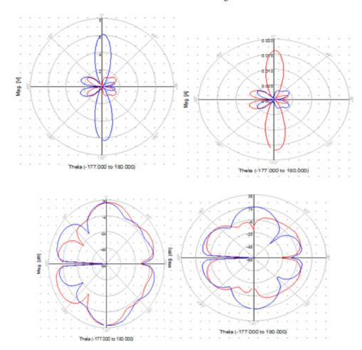
**Figure 7.** E-plane and H-plane polarization, circular polarization and linear polarization for 1st itereation at 3.5 GHz.
