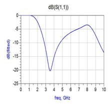
Figure 5(b). Return loss for 1st Iteration.
