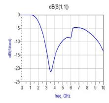
Figure 5(d). Return loss for 3rd Iteration.
