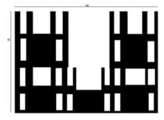
**Figure 4.** Antenna geometry for 3rd iteration.
