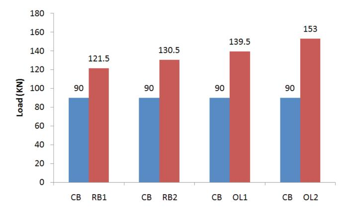
**Figure 6.** Comparison of failure load of control and retrofitted beams.
