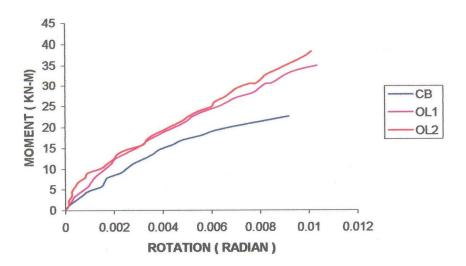
**Figure 8.** Moment vs rotation behavior of overloading beams.
