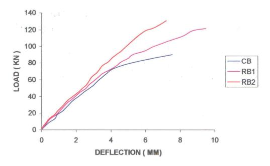
Figure 9. Load vs. deflection behavior of the stressed beams.
