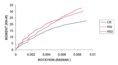
**Figure 7.** Moment vs rotation behavior of the stressed beams.
