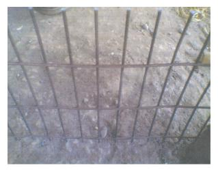
Figure 1. Welded steel wire mesh (a) 2.4 mm dia spacing (25 mm x 25 mm). (b) 3 mm dia spacing (25 mm x 75 mm).
