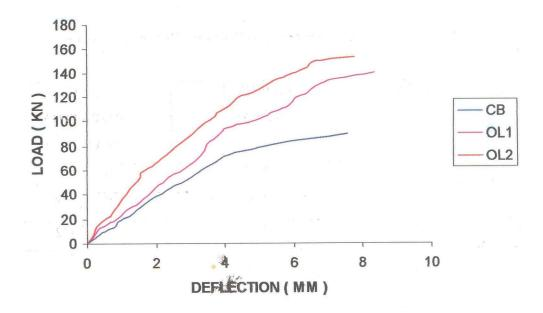
Figure 10. Load vs. deflection behavior of the overloading beams.
