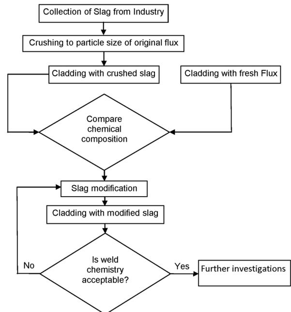
**Figure 1.** Flow diagram of methodology used for recycling the slag.
