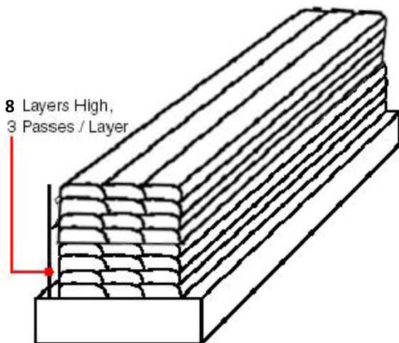
**Figure 2.** Schematic diagram of weld pad.
