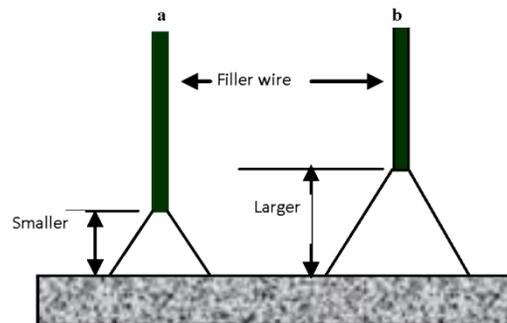
**Figure 5.** Arc shape at (a) Lower arc voltage (b) Higher arc voltage.
