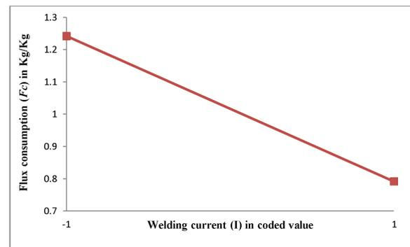
**Figure 6.** Effect of welding current (I) on flux consumption.
