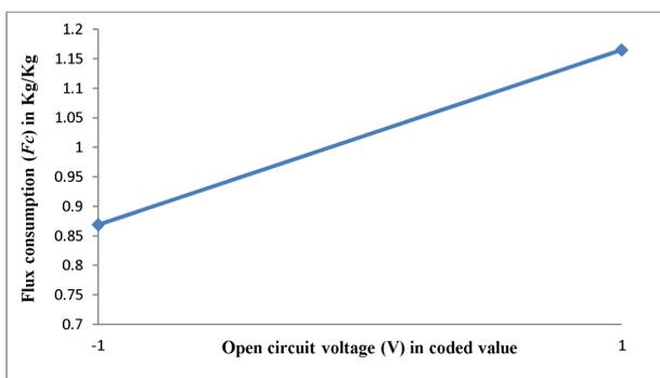
**Figure 4.** Effect of open circuit voltage (V) on flux consumption.
