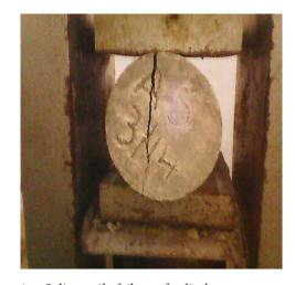
**Figure 4.** Split tensile failure of cylinder.
