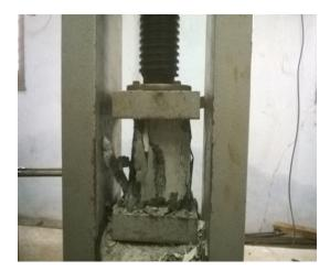
**Figure 3.** Failure of concrete cube during compression load.
