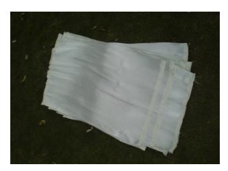
**Figure 2.** GFRP woven roving sheets.
