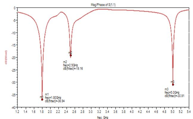
**Figure 5.** S-Parameter calculation of proposed coax fed MIMO antenna at port-1.
