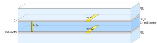
**Figure 2.** Substrate design of coax fed MIMO antenna.
