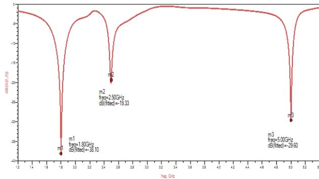
**Figure 6.** S-Parameter calculation of proposed coax fed MIMO antenna at port-2.
