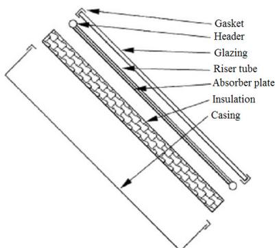
**Figure 2.** Components of a FPC<sup>9</sup>.
