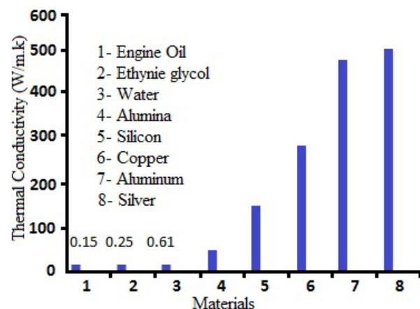
**Figure 4.** The thermal conductivity of the solids and liquids at 300 K<sup>19</sup>.
