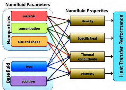
**Figure 3.** The different compounds of nanoparticles soluble and their effects on the various thermophysical properties of Nano fluids<sup>14</sup>.
