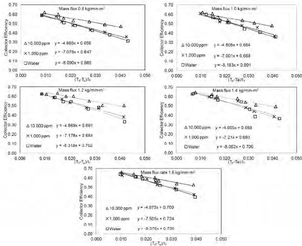
**Figure 5.** The performance of the solar collector at different flow rates and the comparison of the results in the case of silver Nano-fluids with a concentration of 1000 ppm and 10000 ppm, and also the water<sup>18</sup>.
