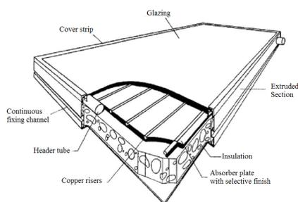
**Figure 1.** Picture of a Flat-plate collector<sup>9</sup>.
