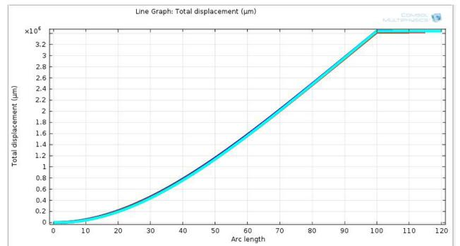
Figure 5e. Arc length vs. total displacement (for varying beam width of range 5 µm to 20 µm at constant length and thickness).
