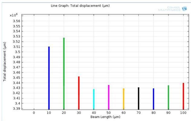
Figure 5c. Beam length vs. total displacement (for varying beam length of range 10 µm to 100 µm at constant beam width and thickness).
