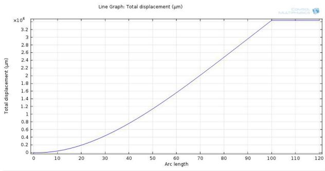
Figure 5b. Arc length vs. total displacement (for 100 µm \* 20 µm \* 0.7 µm).
