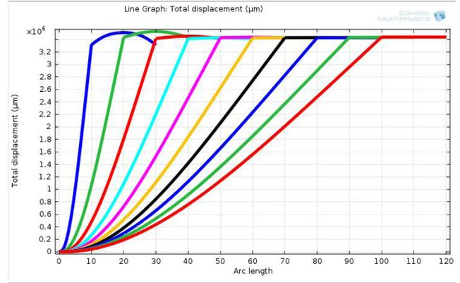
Figure 5d. Arc length vs. total displacement (for varying beam length of range 10 µm to 100 µm at constant width and thickness).
