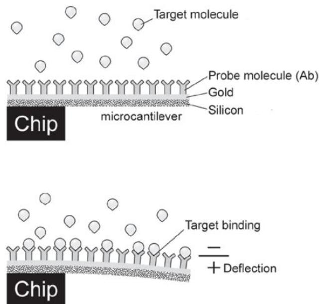
**Figure 1.** Immobilization of antibodies on the cantilever Surface and bending of cantilever after biomolecular recognition.
