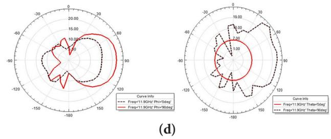
Figure 7. (a) E-plane and H-plane radiations pattern of the antennas at 3.3 GHz. (b) E-plane and H-plane radiations pattern of the antennas at 5.6 GHz. (c) E-plane and H-plane radiations pattern of the antennas at 9.3 GHz. (d) E-plane and H-plane radiations pattern of the antennas at 11.9 GHz.
