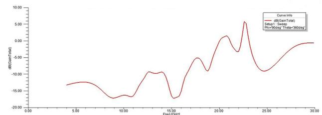
Figure 5. Simulated gain vs frequency of proposed antenna.
