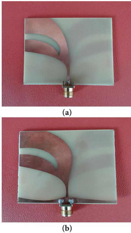
Figure 6. Prototyped AVA with tapered slot edge. (a) Top view. (b) Bottom view.
