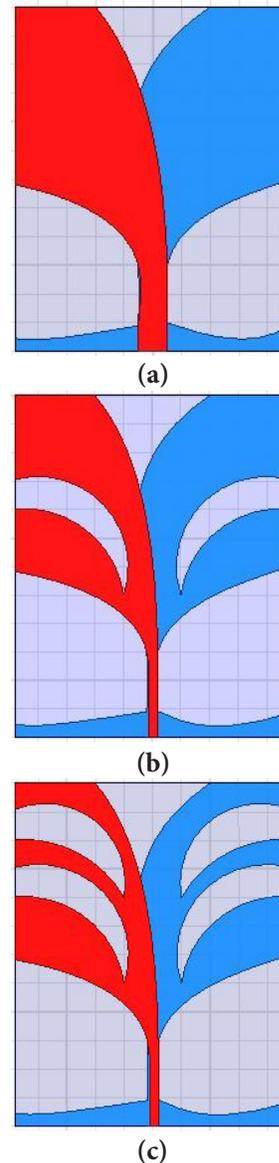
**Figure 1.** Vivaldi antenna iterations. (a) Flared vivaldi base model antenna. (b) Single slotted flared antenna. (c) Double slotted flared antenna.
