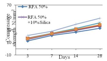
**Figure 3.** Compressive strength of RFA, SFA with addition of silica mortar with 12M NaOH.
