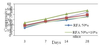
**Figure 5.** Compressive strength of RFA, SFA with addition of Silica with 12M NaOH and Na<sub>2</sub>SiO<sub>3</sub> Alkali activated mortar.
