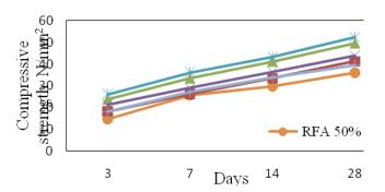
**Figure 4.** Compressive strength of RFA, SFA with addition of Lime with 12M NaOH and Na<sub>2</sub>SiO<sub>3</sub> Alkali activated mortar.
