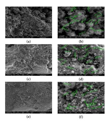
**Figure 6.** SEM images of OPC, RFA and SFA samples. (a) SEM images of OPC at magnification of 50  $\mu$ m. (b) SEM images of OPC at magnification of 5  $\mu$ m. (c) SEM images of RFA at magnification of 50  $\mu$ m. (d) SEM images of RFA at magnification of 5  $\mu$ m. (e) SEM images of SFA at magnification of 50  $\mu$ m. (f) SEM images of SFA at magnification of 5  $\mu$ m.
