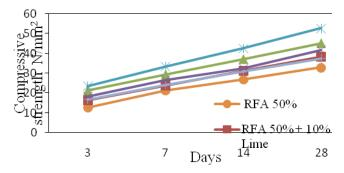
**Figure 2.** Compressive strength of RFA, SFA with addition of lime mortar with 12M NaOH.
