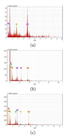
**Figure 7.** (a) EDS spectra of OPC. (b) EDS spectra of RFA. (c) EDS spectra of SFA
