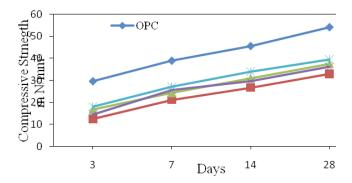
**Figure 1.** Variation of compressive strength of OPC and fly ash geo polymer mortar.
