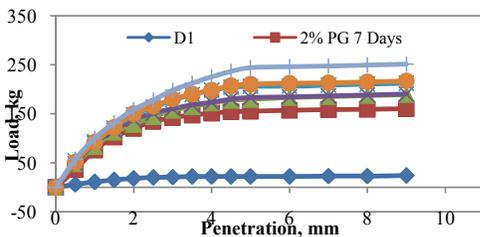
**Figure 3.** Load – penetration curves for untreated and treated D1 soil sample.
