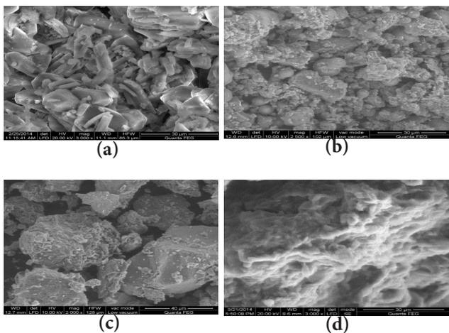
**Figure 5.** SEM micrographs of additives, untreated and treated soil sample. (a) Phosphogypsum. (b) Flyash. (c) Soil D1. (d) Soil sample D1+ 5% flyash +6% phosphogypsum at 28 days of curing.
