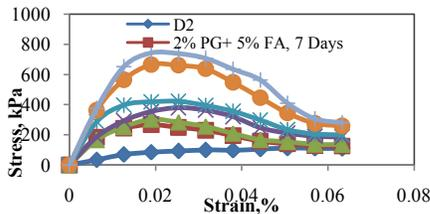
**Figure 2.** Stress-strain curves for untreated and treated D2 soil sample.
