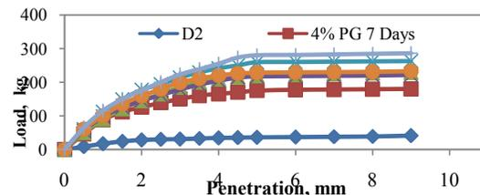
**Figure 4.** Load – penetration curves for untreated and treated D2 soil sample.
