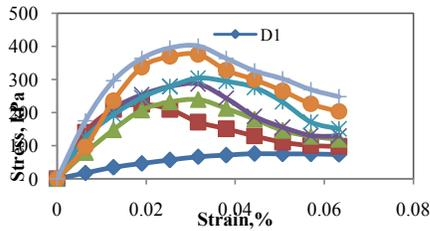
**Figure 1.** Stress-strain curves for untreated and treated D1 soil sample.
