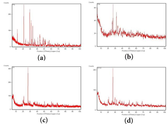
**Figure 6.** XRD results of additives, untreated and treated soil sample. (a) Phosphogypsum. (b) Flyash. (c) Soil D1. (d) Soil Sample D1+ 5% flyash +6% phosphogypsum at 28 days of curing.
