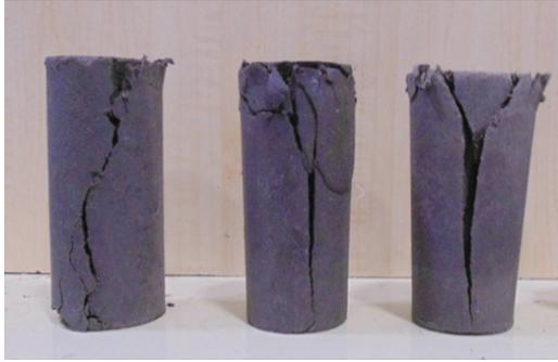
**Figure 3.** Failure pattern of UCC soil specimens with RBI additives for different percentages.
