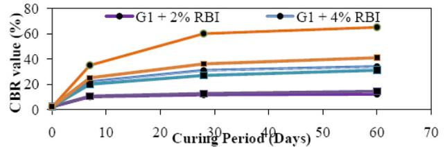
**Figure 5.** Effect of percentage of additive on CBR value for sample G1 and G2.
