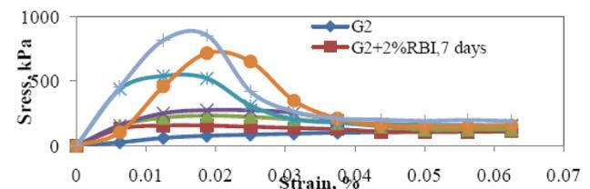
**Figure 2.** Stress – Strain characteristic curve of sample G2 with RBI for different percentages and curing periods.
