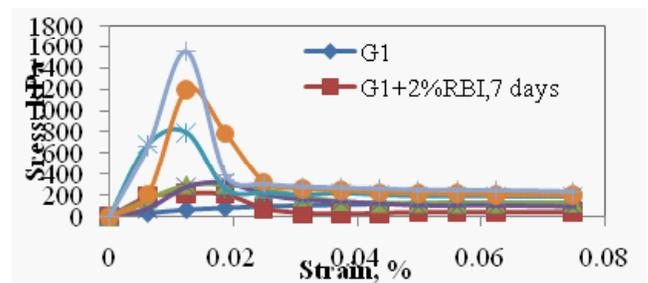
**Figure 1.** Stress – Strain characteristic curve of sample G1 with RBI for different percentages and curing periods.
