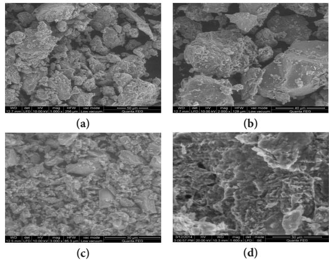
**Figure 6.** Typical SEM micrographs of virgin samples, admixture and treated sample. (a) Sample G1. (b) Sample G2. (c) RBI. (d) Sample G2+ 6% RBI for 60 days curing.
