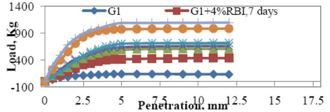
**Figure 4.** Load-penetration curve for soil sample G1 treated with RBI for different curing periods and percentages.
