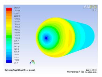
Figure 8. Wall shear stress for V = 18 m/s &N = 900 RPM.
