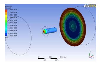
**Figure 10.** Pressure downstream for V = 18m/s & N = 900 RPM.
