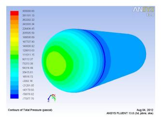
Figure 6. Total pressure on cylinder for V = 18 m/s & N = 900 RPM.
