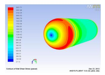
Figure 7. Wall shear stress for V = 18 m/s & without rotation.
