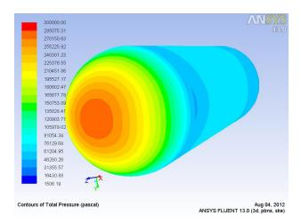
Figure 5. Total pressure on cylinder for V = 18m/s & without rotation.
