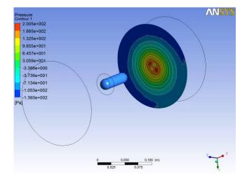
**Figure 9.** Pressure downstream for V=18m/s & without rotation.
