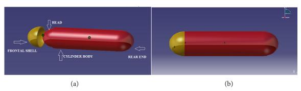
Figure 1. Axisymmetric body with frontal shell (a) Exploded view (b) Assembled view.
